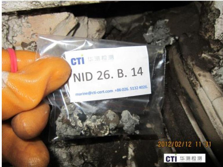
Picture: Cable penetration detected containing asbestos from newbuilding ship
